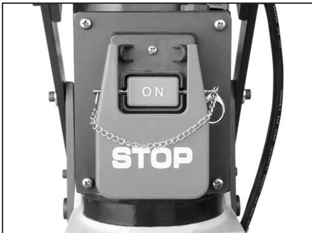
Figure 16. Switch disabling pin installed.
