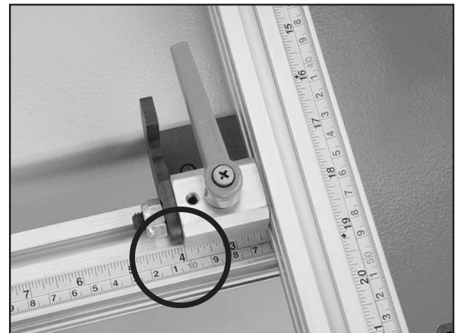
Figure 24. Distance of 4" of the longitudinal fence from boring bit centers, as read on the cross fence scale.
