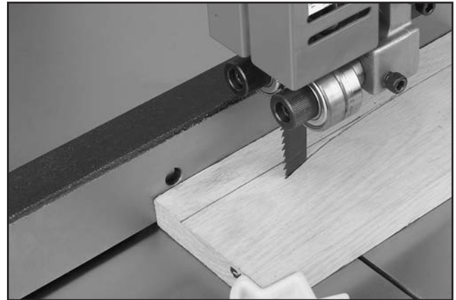
Figure 64. Blade leading away from line of cut.
