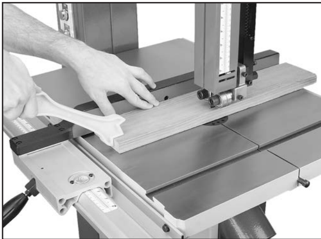
Figure 40. Ripping with a push stick.
