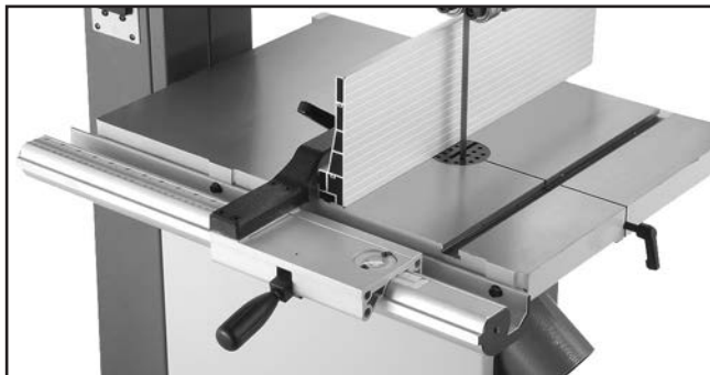
Figure 12. Correctly installed fence.
