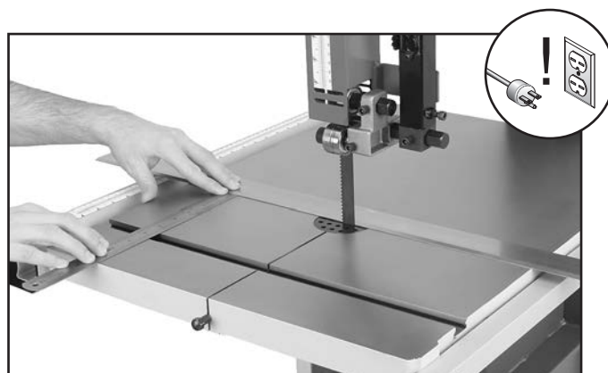
Figure 27. Measuring for miter slot to be parallel with blade.
