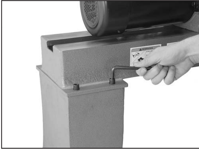
Figure 12. Securing lathe assembly to supporting legs.
