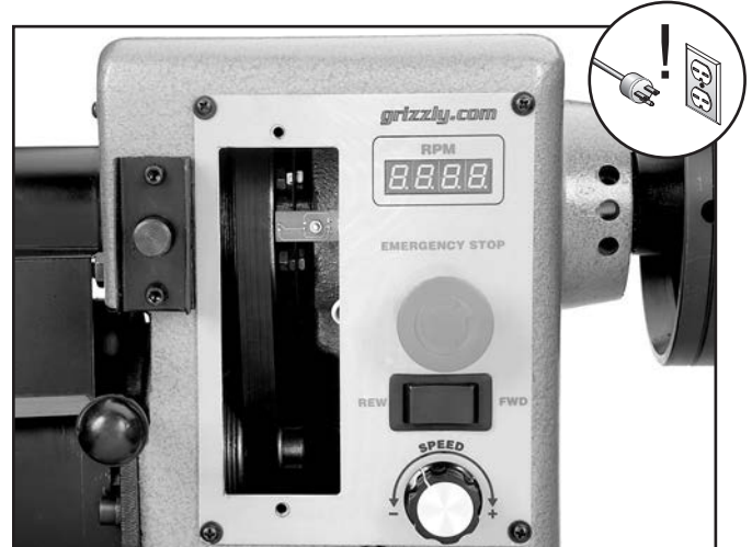
Figure 32. Belt access panel removed.
