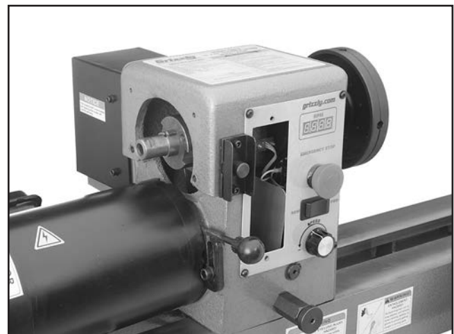
Figure 57. Headstock with spindle handwheel and belt access panels removed.
