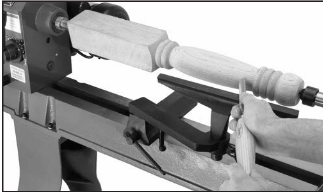
Figure 42. Typical spindle turning operation.
