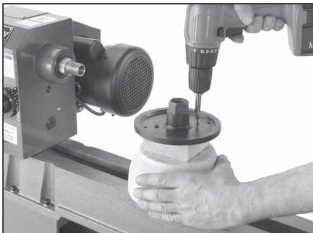
Figure 47. Typical attachment of faceplate to workpiece (shown with backing block).
