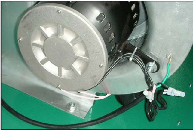
Figure 26. Left motor wiring.
