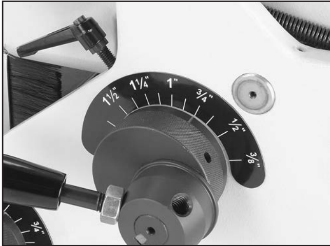
Figure 19. Clamp set to \frac{3}{4} " , as indicated on the scale.
