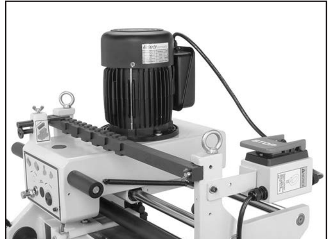
Figure 5. Switch moved for access to the eye bolt.
