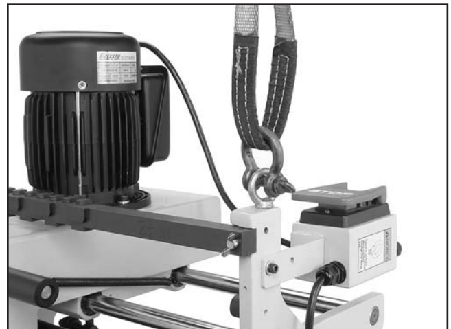
Figure 6. Lifting machine from eyes.
