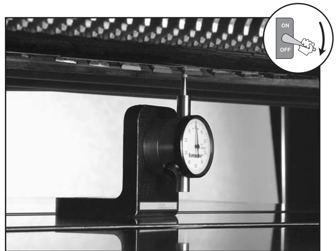
Figure 34. Finding BDC with the Rotacator.
