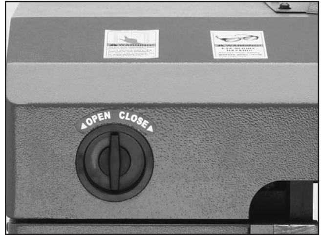
Figure 19. Headstock cover latch in closed position.
