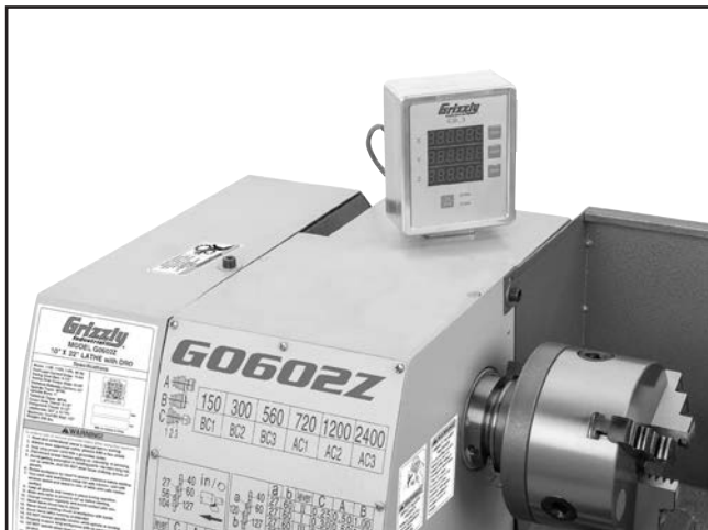
Figure 9. DRO magnetically mounted on lathe headstock.
