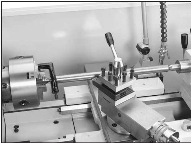
Figure 48. Example photo of a workpiece mounted between the centers.
