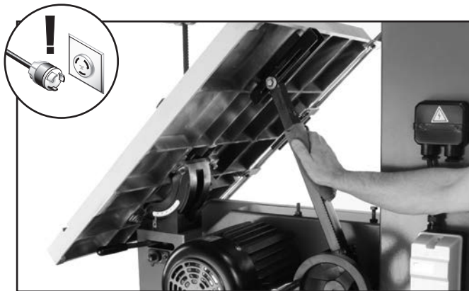
Figure 73. Example of lubricating table tilt rack and pinion assembly.
