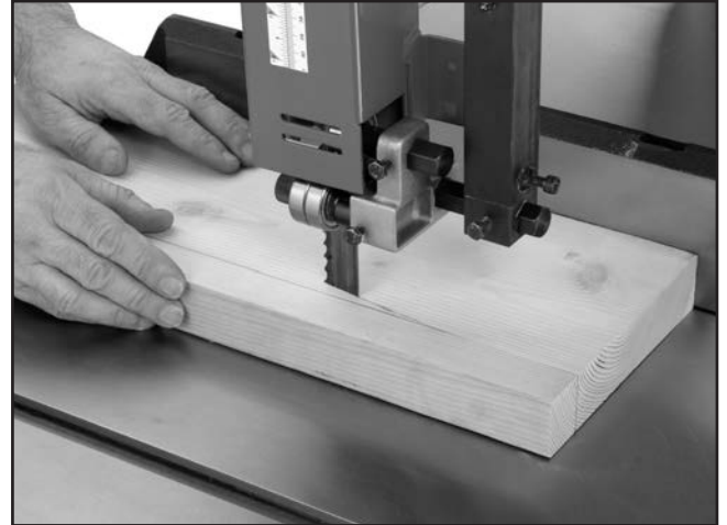
Figure 59. Blade leading away from line of cut.
