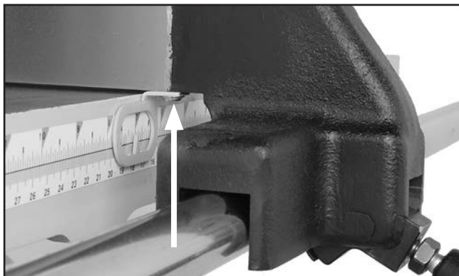
Figure 42. Fence pointer adjustment screw.
