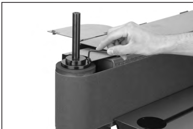
Figure 19. Tightening cap screws.
