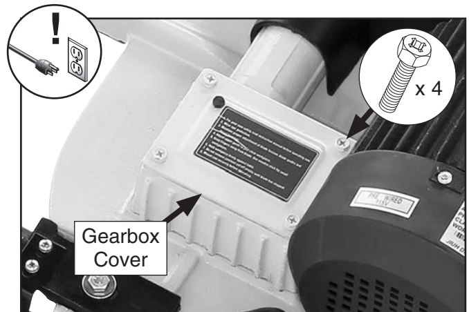
Figure 69. Location of gearbox cover and bolts.
