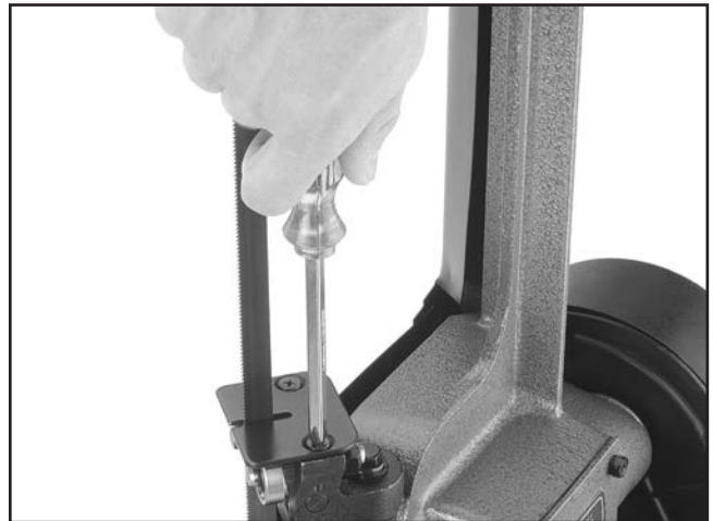
Figure 56. Location of flat head screws holding blade guide cover.
