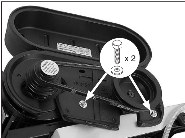
Figure 19. Pulley cover installed.
