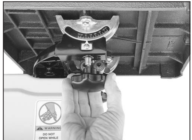
Figure 17. Securing table to the trunnion.
