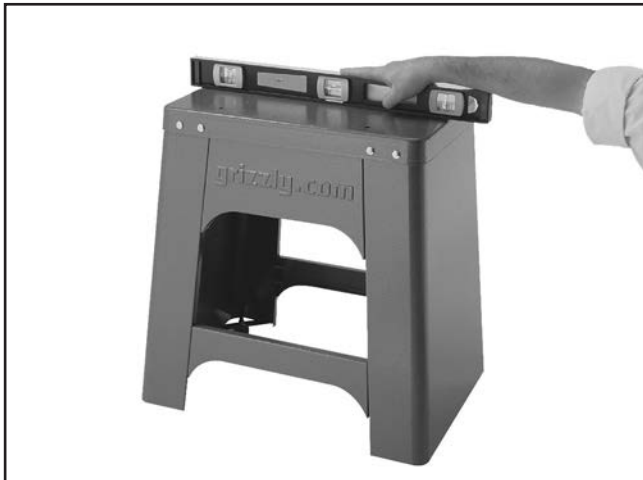
Figure 12. Leveling the stand.
