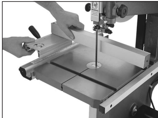
Figure 20. Placing the fence onto the rails.
