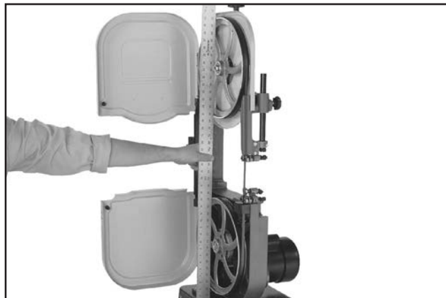
Figure 62. Checking if the wheels are coplanar.
