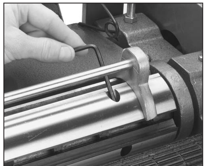
Figure 8. Adjusting knife height.
