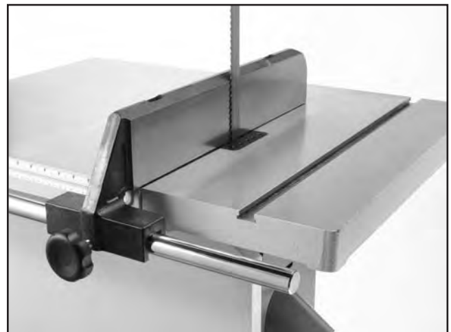
Figure 19. Fence flush with blade.
