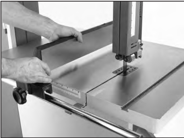
Figure 11. Installing fence onto rail.
