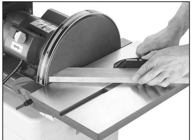
Figure 19. Disc sanding with miter.
