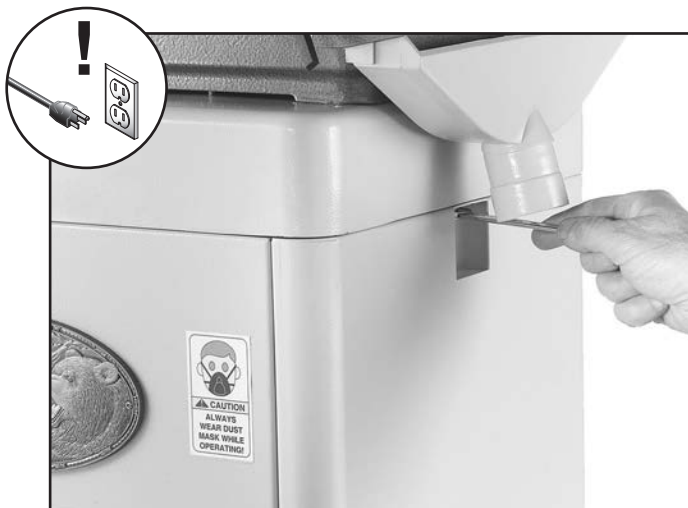
Figure 6. Cabinet hole location.
