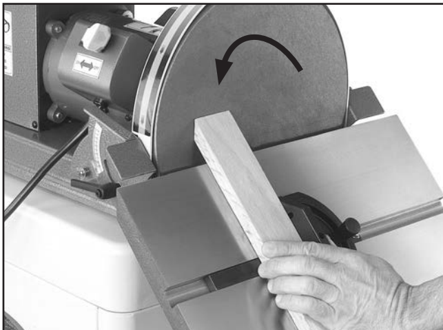
Figure 18. Disc sanding with table tilted.
