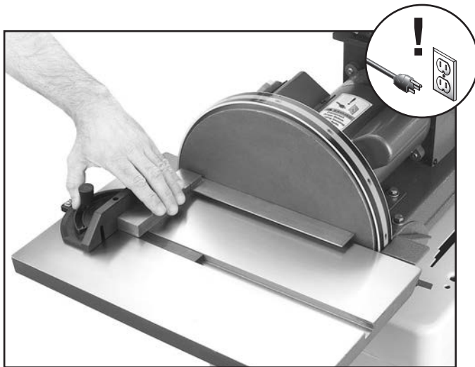
Figure 14. Squaring miter gauge to disc.
