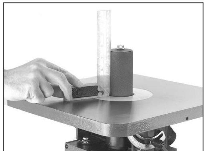
Figure 10. Squaring the table and spindle.
