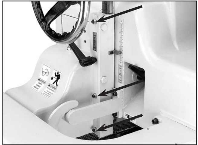
Figure 41. Gib adjustment setscrews.
