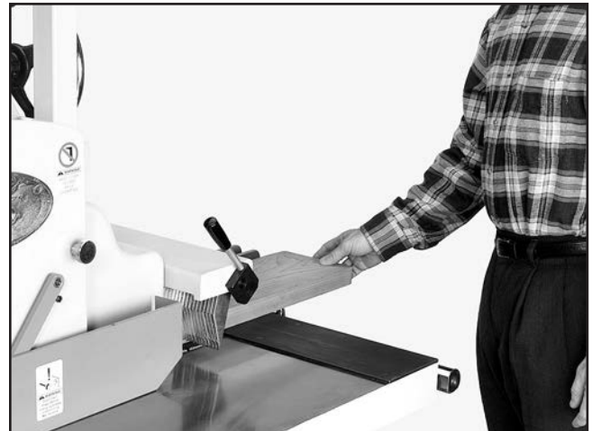
Figure 31. Rip cutting operation. The operator is standing to the side of the workpiece to avoid injury in the event of kickback.
