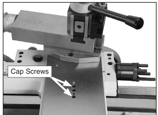
Figure 62. Cross slide backlash adjustment socket head cap screws.
