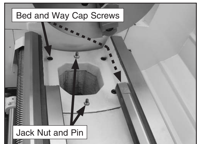
Figure 19. Lathe gap and pin arrangement.
