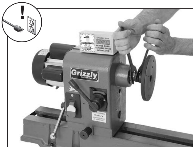
Figure 25. Tightening the faceplate onto the spindle.
