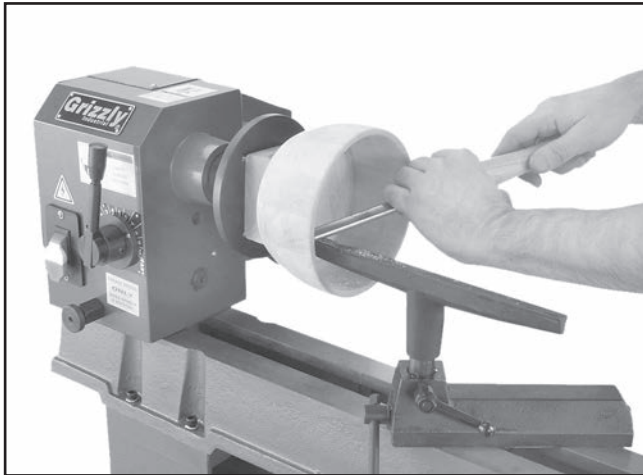
Figure 36. Typical faceplate turning operation.
