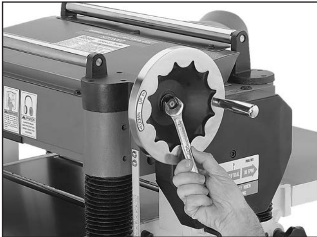
Figure 9. Installing the table height handwheel.
