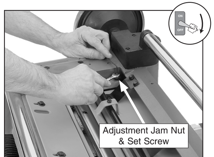
Figure 40. Example of adjusting the pressure bar height.
