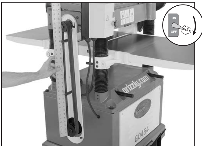
Figure 34. Checking pulley alignment.
