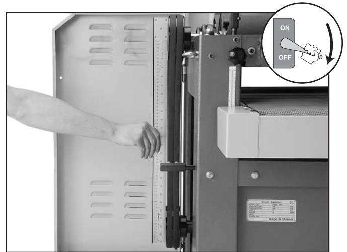
Figure 45. Checking pulley alignment with a straightedge.
