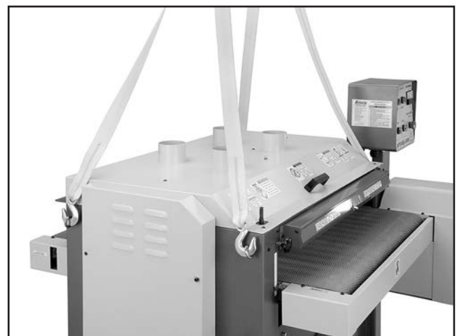
Figure 13. Lifting the sander.
