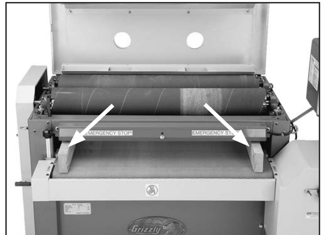
Figure 64. Gauge blocks in position for adjusting the pressure roller height.
