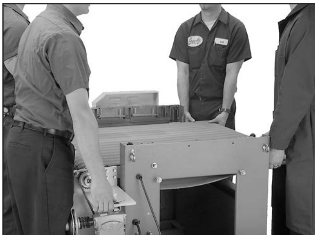
Figure 75. Lifting the table off of the drum sander cabinet with four people.
