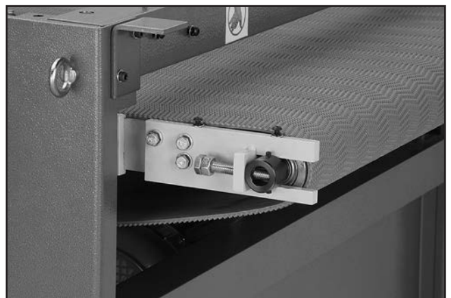
Figure 73. Conveyor belt loosened at the rear adjustment.
