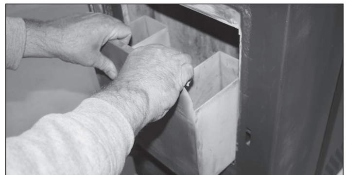
Figure 34: Dump Ash Pan
