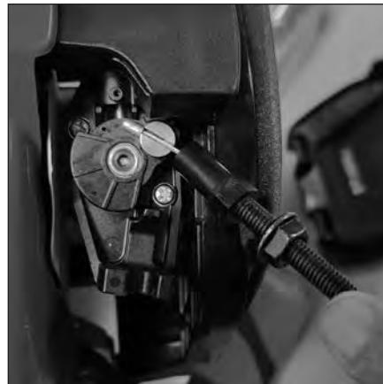
After the throttle stop has been installed, position the cable in the silver throttle swivel as shown above
