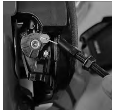
Pull the cable so the tip is secure within the swivel slot
