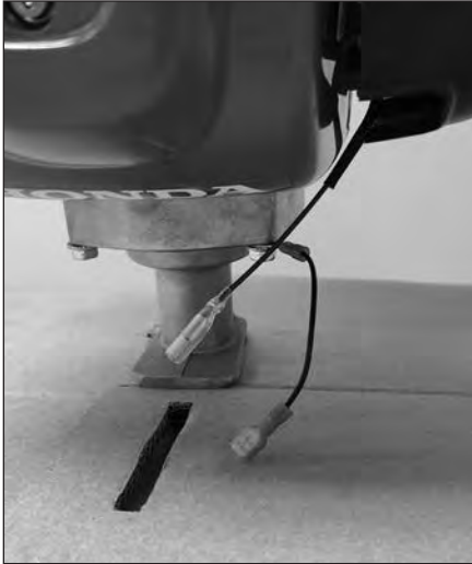
Throttle connections on XP tiller engine
