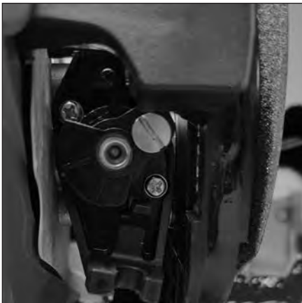
Engine throttle assembly with air cleaner cover removed
