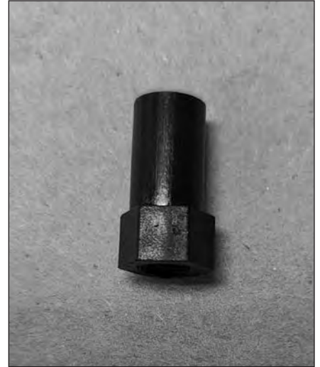
Throttle Stop oriented in the correct position for installation
