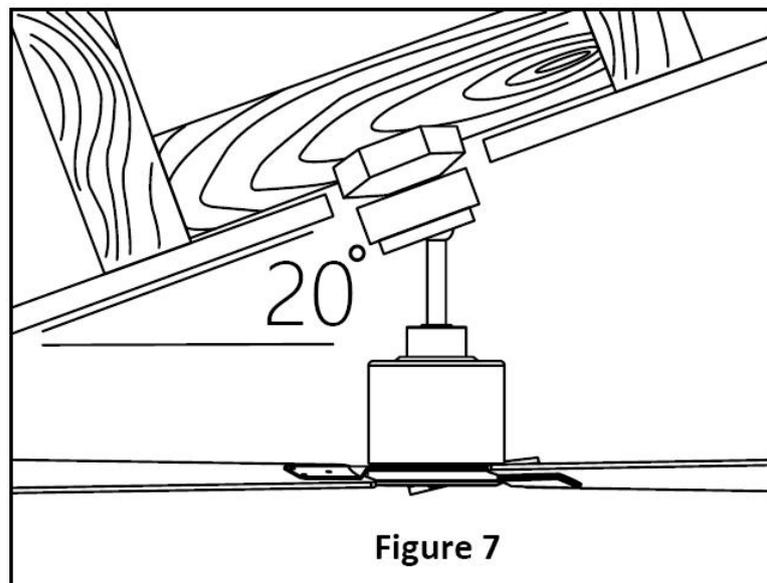
**3****Installing Down rod.**
