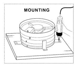
6. Carry the Gable mount Ventilator and plywood assembly into the attic, position it behind the shutter and screw it to the gable framing.
