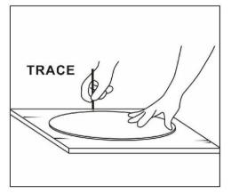
4. Use a sabre saw to cut out the airway on the plywood for mounting the gable mount ventilator.
