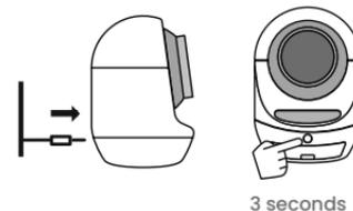
Plug power adapter into an outlet and wait for a beep. Then turn the unit on by pressing the power button for 3 seconds. The drum will rotate and light will flash.
