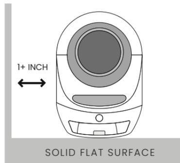
Place unit on a flat even surface to ensure all sensors function properly. **Do not place unit directly on carpet or rugs.**
