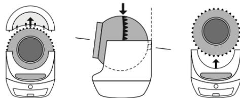
Verify the rotating drum is secure, as it may have shifted during shipping. Drum should be seated evenly in the gear track with spindle aligned in holder.
