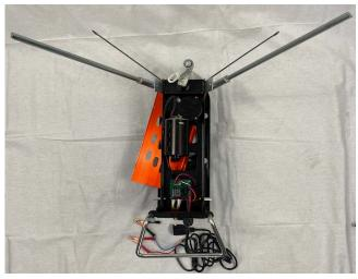
STRAIGHTEN OUT THROWING ARM (ONLY MOVES ONE DIRECTION) FEED THREADED SPADE BOLT WITH SPRING (ID: C) THROUGH HOLE, HOOK SPRING TO METAL SLOTTED TAB THAT DRIVES THROWING ARM, THREAD ON TENSION KNOB (ID: D)
