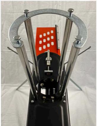
FEED ORANGE SAFETY RING TUBING (ID: I) THROUGH SAFETY RING MOUNT ARMS (ID: H) AND THEN SLIDE ENDS OF TUBING OVER STRAIGHT HEX BOLTS FOR SAFETY RING (ID: O)
