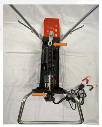
FLIP CLAY PIGEON THROWER OVER AND PUT THE 4 CLAY PIGEON STACK RODS (ID: J) ONTO MALE KNUBS (NOTE THREADED HOLE AT TOP TO FASTEN CLAY STACK HORSESHOE (ID: K) MOUNT ALL 4 RODS
