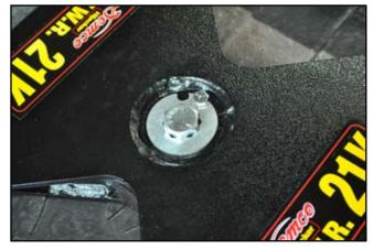
**3.** Once the B&W hitch pin fully returns into the adapter, tighten the top bolt to 20-25 ft lbs. and use the bolt retainer with 1/4" bolt to hold bolt into place as shown.
