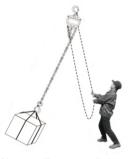
8. Never pull at an angle, be sure hoist and load are in a straight line.
