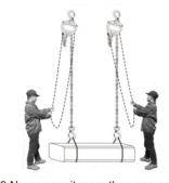
9. Never permit more than one operator to pull on a single hand chain at one time.
