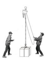
5. Never lift a load unless chain is properly seated in chain wheel(s).
