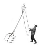
8.Never pull at an angle,be sure hoist and load are in a straight line.
