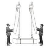
9.Never permit more than one operator to pull on a single hand chain at one time.
