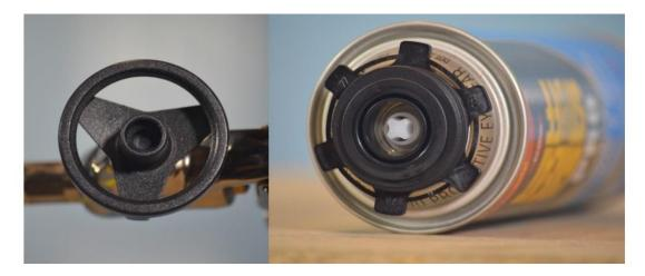
A protective cap ships with the can, remove it. You will see a plunger button within the collar. When the can is attached to the gun, the plunger depresses, foam flows into the gun. The can attaches to the gun by simply screwing into the basket on the gun. In order to expand and cure, the foam needs to react with air and moisture (in the air). As long as the foam is in the can or within the gun, air doesn't reach it and it does not cure.
