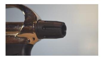
The knob on the end of the gun controls the flow of foam.
