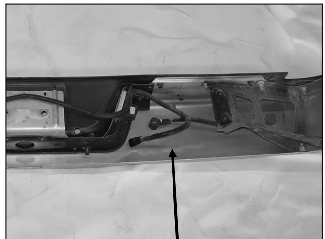
(Fig 10) Unplug and remove the factory sensors and wiring harness. Note location of each sensor for proper reinstallation
