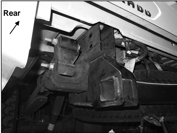
(Fig 3) Remove bumper and brackets
