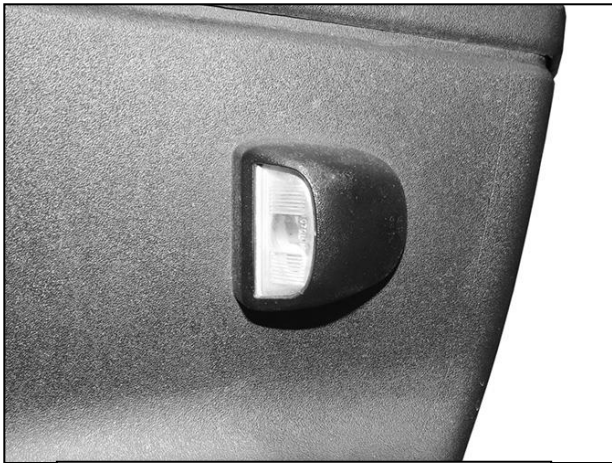
(Fig 10) Remove license plate lights (2011-14 model pictured)
