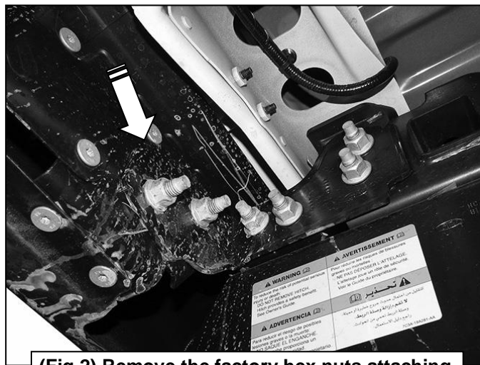
(Fig 2) Remove the factory hex nuts attaching the bumper to the brackets (arrow)
