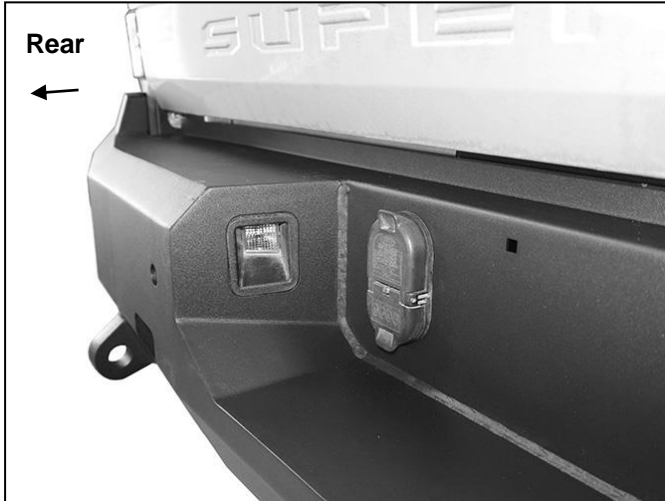
(Fig 11) Install wiring harness, trailer plug and license plate lights before installing Bumper
