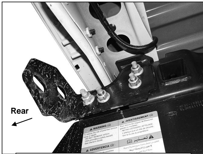
(Fig 3) Remove bumper bracket from frame
