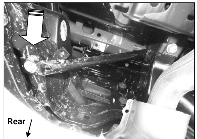
(Fig 4) Remove the bolts attaching the outer bumper supports to the bottom of the bumper (arrow)
