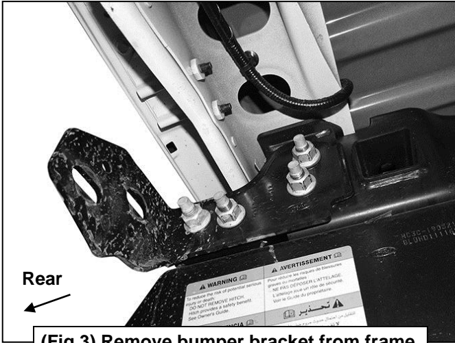
(Fig 3) Remove bumper bracket from frame
