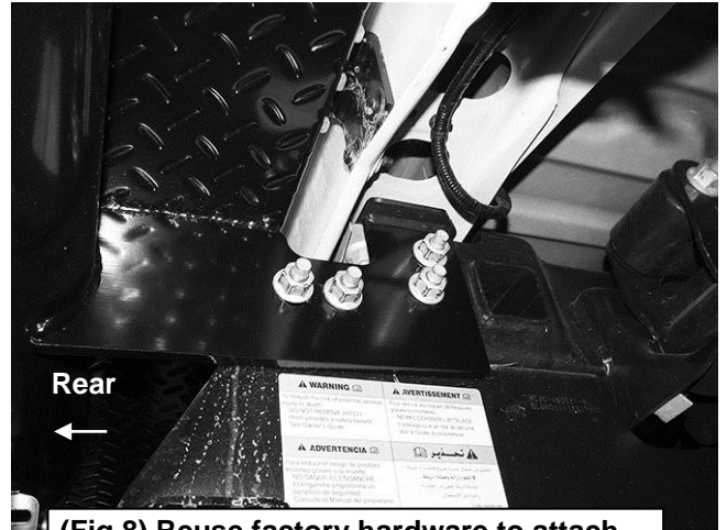
(Fig 8) Reuse factory hardware to attach passenger/right Bumper to side of frame
