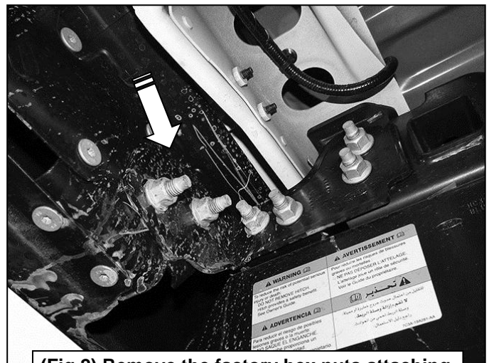
(Fig 2) Remove the factory hex nuts attaching the bumper to the brackets (arrow)
