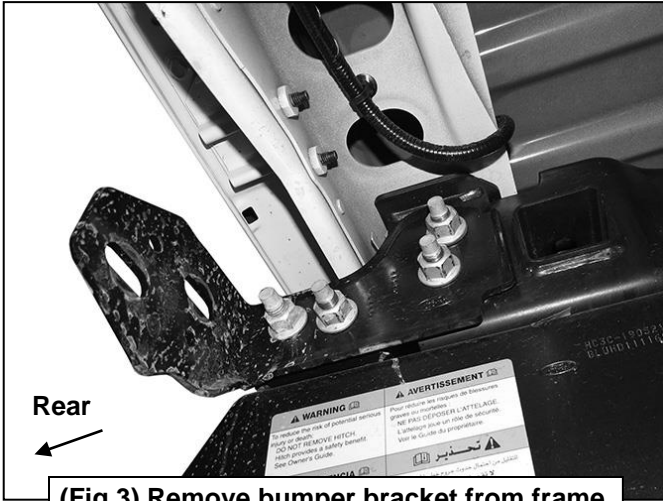
(Fig 3) Remove bumper bracket from frame
