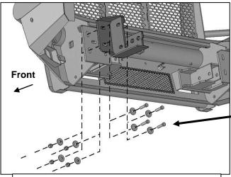
(Fig 10) Attach Bumper to driver/left Bracket
