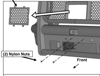
(Fig 12) Attach License Plate Bracket to Bumper
