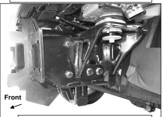
(Fig 3) Reuse factory hardware to attach (1) Frame Bracket to the outside of the frame (driver/left side pictured)
