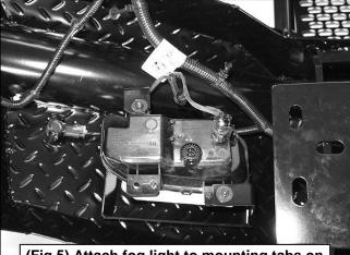
(Fig 5) Attach fog light to mounting tabs on back of Bumper (driver/left side pictured)
