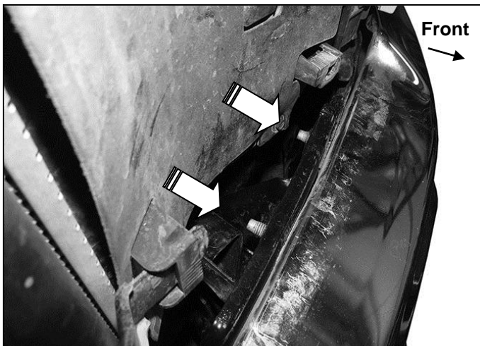
(Fig 3) Remove driver side top bumper hardware
