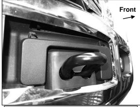
(Fig 1) Remove cover over bumper bolts (2017-19 model year pictured)
