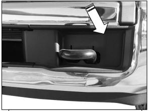
(Fig 2) An opening in the plastic covers must be cut for reinstallation (2020-on model pictured)
