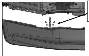
Hold air dam up against bottom of Brackets (dashed line for reference). Mark location of Bracket onto top of air dam (arrows)
