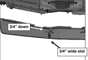
(Fig 15) Driver side-back of "short" air dam illustrated. All measurements are for reference and example only, check all measurements before cutting air dam.
