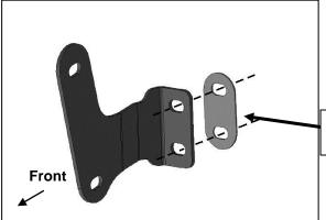
(Fig 5) On 2017-19 models only, attach driver/left Frame Bracket to Spacer and bumper. Do not install Bracket without Spacer on 2017-19 model years
