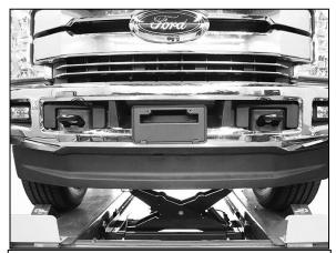
(Fig 7) Remove plastic air dam from bumper
