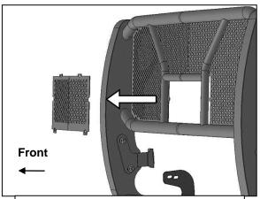
(Fig 16) On models with grille mounted camera, remove center screen
