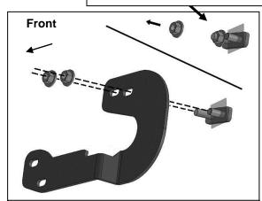
(Fig 9) Driver/left Lower Bracket illustrated. Reuse factory hardware to attach Bracket to side of frame and frame extension
