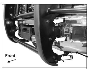
(Fig 12) Attach Grille Guard to outside of Brackets (arrows)
