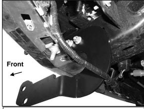
(Fig 11) Driver/left Lower Bracket pictured. Reuse factory hardware to attach Bracket to side of frame and frame extension
