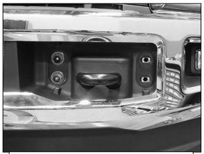
(Fig 3) Remove outer bumper bolts only
