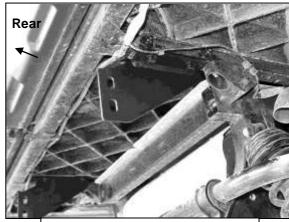
(Fig 9) Frame Brackets installed
