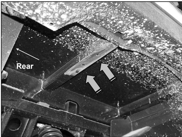
(Fig 1) Locate the Passenger/Right mounting location under the bed
