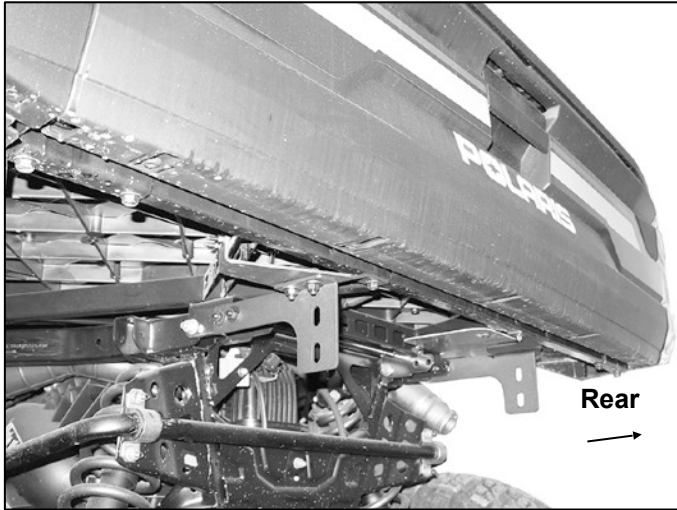
(Fig 7) Brackets installed
