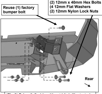
(Fig 9) Driver/left side without hitch illustrated
