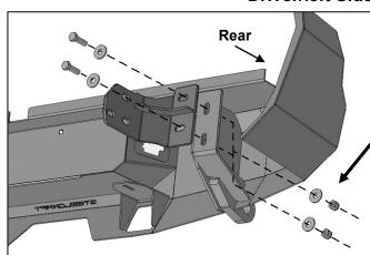
(Fig 6) Attach Driver/Left Frame Bracket to back of Bumper. Leave hardware loose at this time
