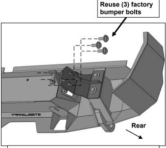
(Fig 11) Driver/left side Bumper Bracket attached to frame and Support Bracket (model with factory HD hitch and tow package)
