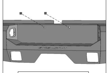
(Fig 12) Push plastic plugs into holes in Bumper for license plate
