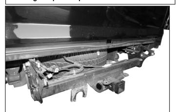
(Fig 5) Models with receiver hitch only, remove bumper but leave receiver hitch attached
