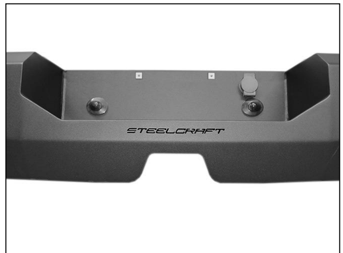
(Fig 6) Push plastic plugs into holes for license plate. Install license plate lights and spare tire access lock
