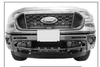
(Fig 5) Remove center plastic bumper cover and license plate
