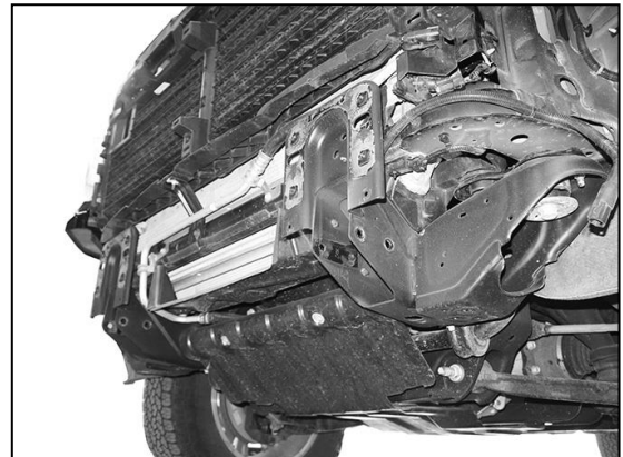
(Fig 7) Bumper brackets removed
