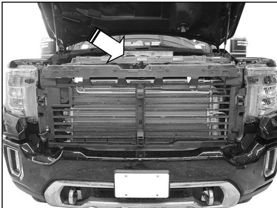
(Fig 3) Reattach hood release lever. Disconnect wire harnesses leading to bumper
