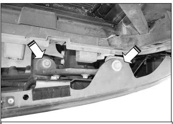
(Fig 4) Remove bumper bolts (pictured from above)
