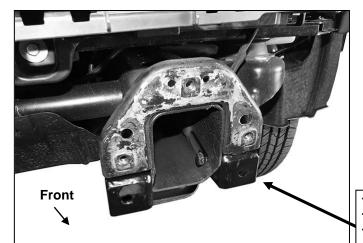
(Fig 9) Attach Support Brackets to frame using factory holes for tow hooks. Driver side pictured
