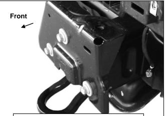
(Fig 5) Remove inner bumper brackets and tow hooks, reinstall plastic grille
