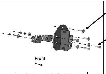
(Fig 10) Attach Driver/Left Mounting Bracket to mounting plates on end of frame and L/R Support Brackets
