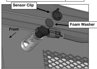
(Fig 14) Slide sensor into sleeve, insert Foam
