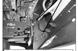
(Fig 17) Driver/Left side of Bumper attached to Bracket (pictured from behind Bumper)
