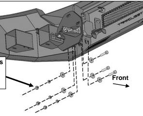
(Fig 16) Attach Driver/Left side of Bumper to Bracket
