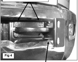
IMPORANT: To prevent damage to the bumper and/or Frame Mounting Brackets, do not allow the Brackets to come in contact, top or bottom, with the steel bumper
