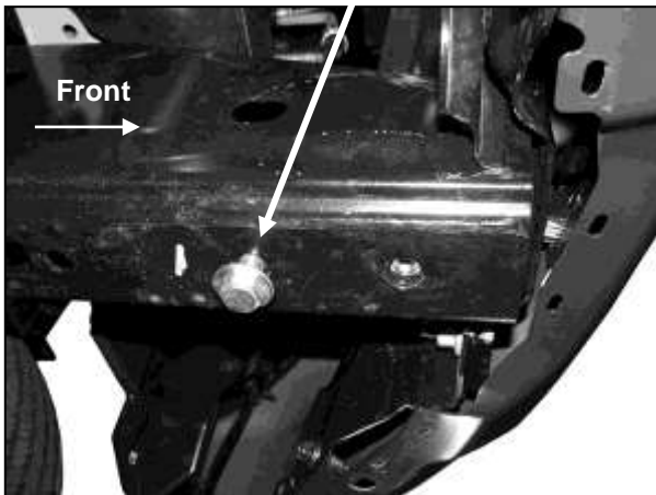
(Fig 19) Use 12mm Hex Bolts to line up and hold the Nut Plate in place
