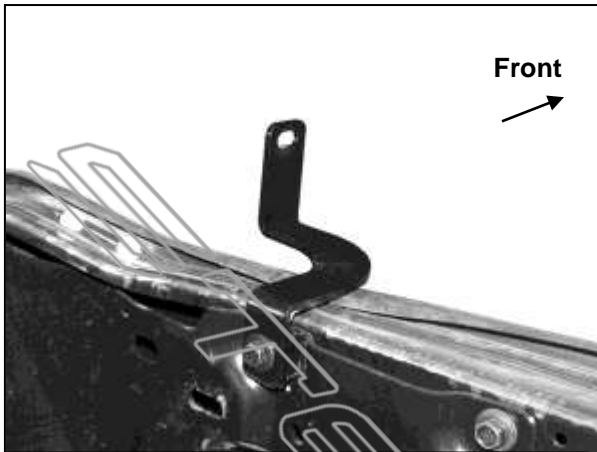
(Fig 9) 2018-20 models: Attach Top Support Bracket to back of bumper bracket
