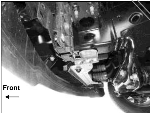
(Fig 11) Active air dam removed
