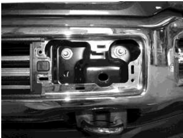
(Fig 3) 2018-20 models: From behind bumper, locate and remove bolts attaching bottom of bumper to bumper brackets. From front of bumper, remove bumper pad to locate and remove hex nuts and remove bumper.
