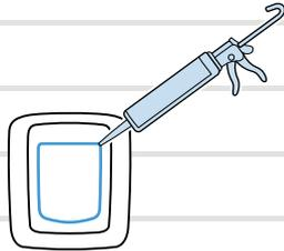
**EN** Apply exterior-grade caulk around the edge of the pet door tunnel where it meets the exterior frame.
