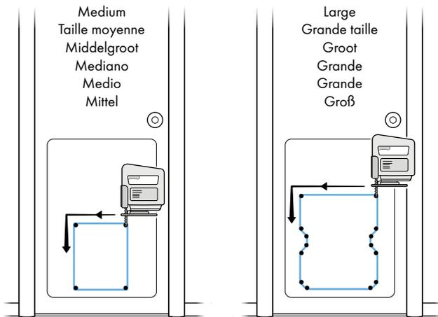
**EN** Using a jigsaw, cut between the holes you just drilled, along the cutting line. Make sure your jigsaw blade is designed to cut metal and is at least 1 inch (25 mm) longer than the thickness of your door.
