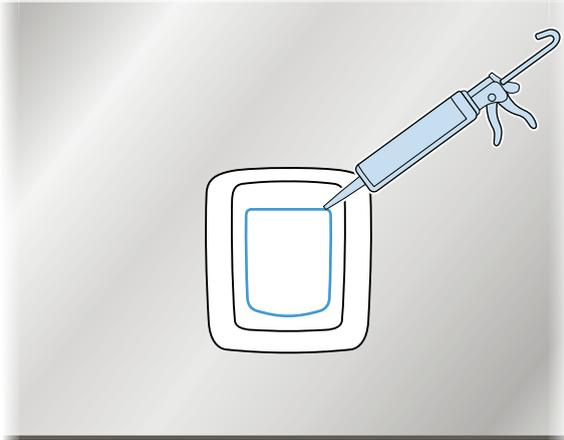
**EN** Apply exterior-grade caulk around the edge of the pet door tunnel where it meets the exterior frame.
