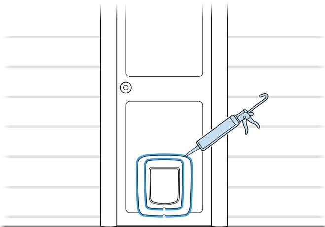
**EN** On the exterior side of the door, apply exterior-grade caulk around the edges of the installation adaptor and the exterior frame, making sure to leave the weep holes open.
