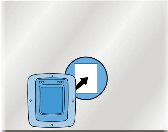
**EN** Insert the tunnel of the interior frame through the middle of the installation adaptor. The smooth side of the installation adaptor should face the front.
