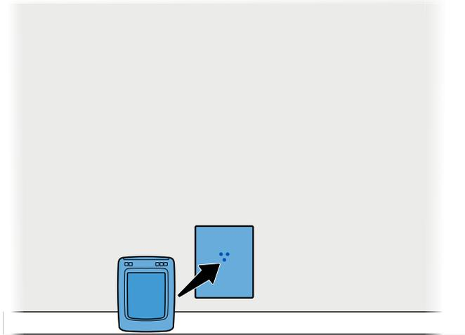
**EN** If you used the template for wall installation (without metal), insert the interior frame of the pet door into the opening to check the fit.
