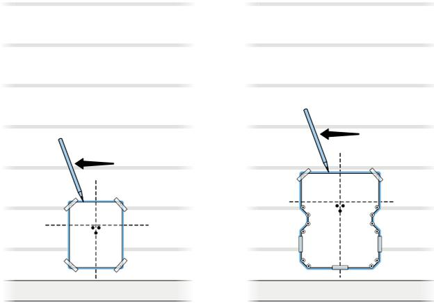
**EN** You are now ready to work from the exterior wall. Line up the three holes in the cutting template with the three holes you drilled through the wall. Make sure the template is level and then tape it into position.
