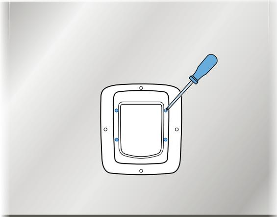
**EN** On the exterior side of the glass, line up the second installation adaptor and exterior frame with the pet door tunnel.
