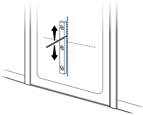
**EN** Draw a vertical line where you want the center/centre of the pet door to be. If your door has inset panels, consider how best to position the pet door to avoid gaps between the pet door frames and the door.
