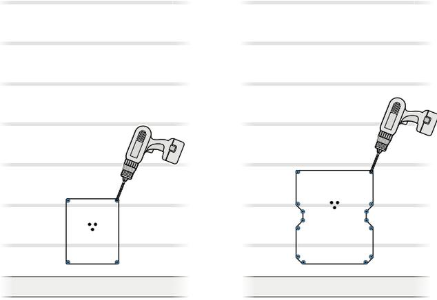
**EN** Drill 1/2-inch (12 mm) holes through the exterior wall, just inside the corners of the cutting line.
