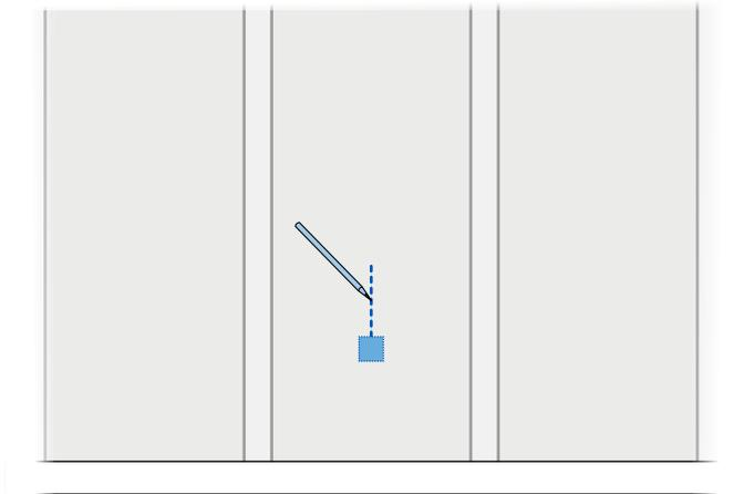
**EN** Choose a location for the SmartDoor™. It should be in a section of wall that is easily accessible by your pet and away from any electrical wiring or plumbing.
