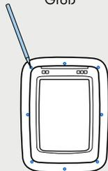
**EN** Insert the interior pet door assembly (interior frame with attached installation adaptor and tunnel extensions) into the opening in the interior wall.
