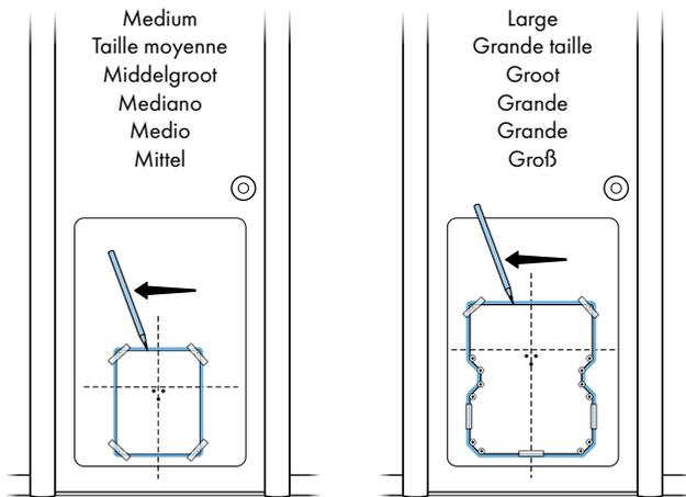
**EN** Once you are satisfied with the placement of the template, use a pencil to trace the outside edge of the cutting template. Remember to connect the corners.
