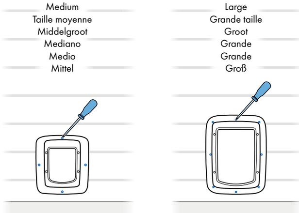
**EN** Replace the exterior pet door assembly and secure it to the exterior wall with appropriate hardware for your construction (not included).
