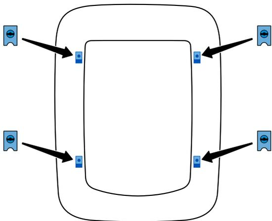
**EN** Place the second installation adaptor on a flat surface, smooth side up.
