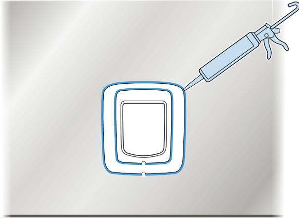
**EN** On the exterior side of the glass, apply exterior-grade caulk around the edges of the installation adaptor and the exterior frame, making sure to leave the weep holes open.
