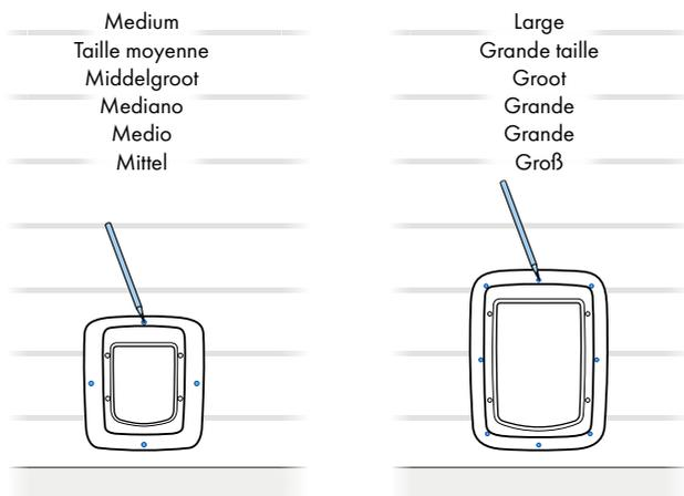
**EN** On the exterior side of the wall, line up the exterior pet door assembly (exterior frame with attached installation adaptor) with the tunnel of the pet door.
