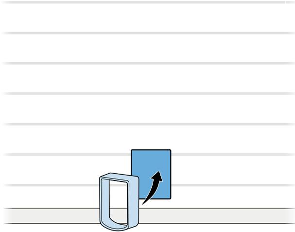
**EN** If you used the template for wall installation (without metal), insert a tunnel extension into the opening to check the fit.
