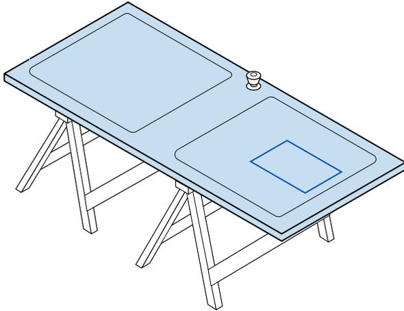
**EN** If desired, remove your door from its hinges and place it on a raised, level surface, such as two sawhorses. The interior side of the door should face up.
