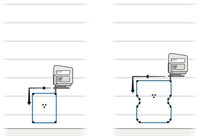
**EN** Using a jigsaw, cut the exterior wall between the holes you just drilled, along the cutting line.
