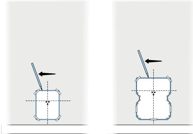
**EN** Trace the outside edge of the cutting template, making sure to connect the corners.
