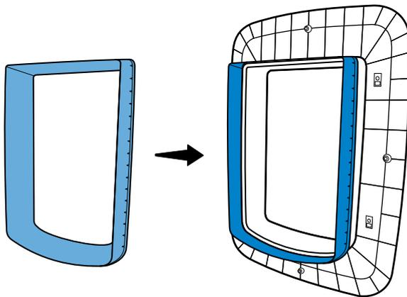
**EN** Connect a tunnel extension to the pet door by fitting the lip of the tunnel extension over the tunnel of the pet door.
