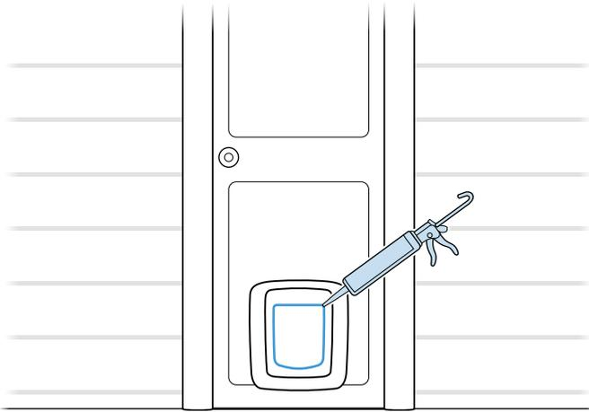
**EN** Apply exterior grade caulk around the edge of the pet door tunnel where it meets the exterior frame.
