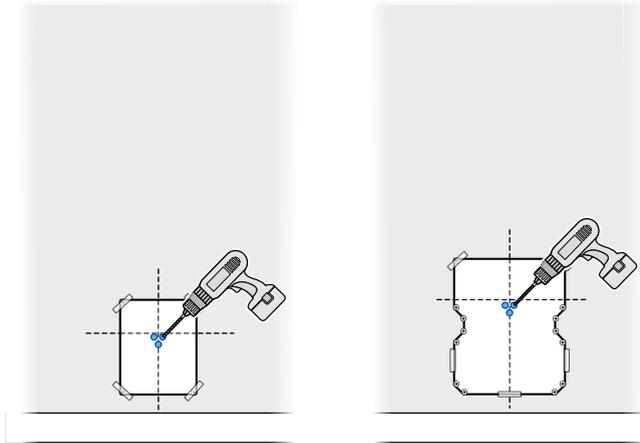
**EN** Once you are satisfied with the placement of the cutting template, use a long drill bit to drill three holes through the center/centre locator holes on the template and all the way through the interior and exterior surfaces of the wall.
