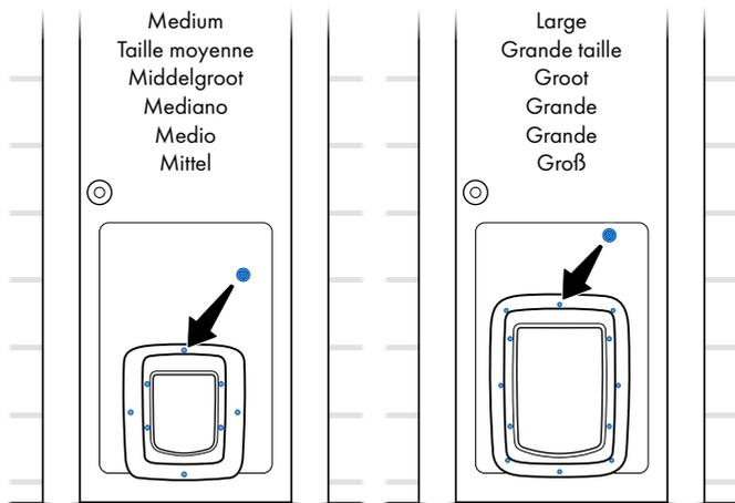
**EN** On the exterior side of the door, insert blanking plugs into the holes in the exterior frame. These blanking plugs were supplied with the pet door.
