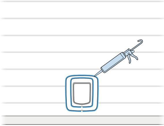
**EN** On the exterior side of the wall, apply exterior-grade caulk around the edges of the installation adaptor and the exterior frame, making sure to leave the weep holes open.
