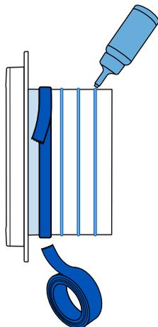
**EN** Once you are satisfied that you have connected the appropriate number of tunnel extensions, remove the tunnel extensions from the pet door and use permanent glue to attach the tunnel extensions to one another.
