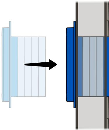
**EN** Test fit the interior frame (with installation adaptor and tunnel extensions attached) in the opening. The last tunnel extension needs to protrude from the wall by at least 1 1/4 inches (33 mm).
