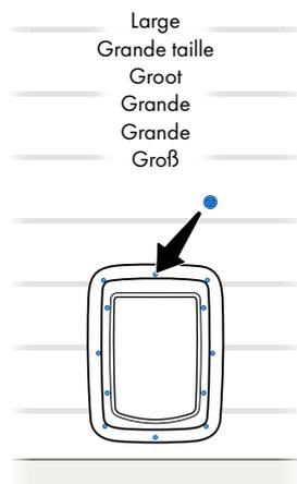
**EN** On the exterior side of the wall, insert blanking plugs into the holes in the exterior frame. These blanking plugs were supplied with the pet door.
