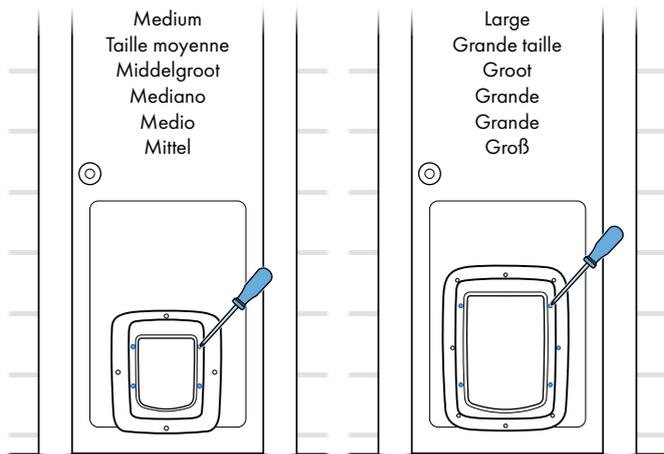
**EN** Using a manual #2 Phillips (crosshead) screwdriver, tighten the screws just until the frames are attached.
